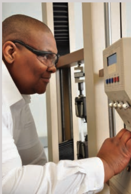
Figure 6 Lab technician Aaron Walker tests a Type I specimen bar in tension mode to obtain the material's tensile strength and elongation values.
