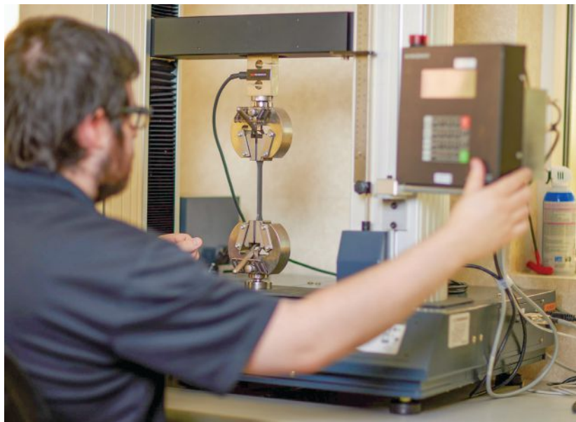
An injection molded sample is tested for tensile properties at AGS. Source: AGS Technology
