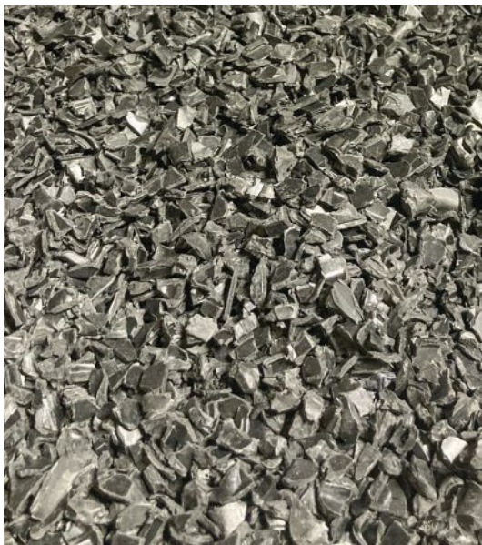
Black nylon regrind as received by AGS Technology. Source: Matt Stonecash
